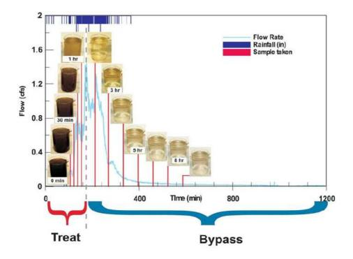
Figure 1: Stormwater First Flush Contaminant Characterisation
