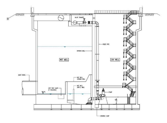
Figure 6: Pump station wet well/dry well arrangement
