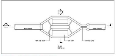
Figure 5-4 Typical grit trap arrangement
