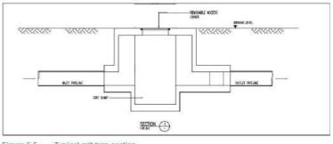
Figure 5-5 Typical grit trap section
